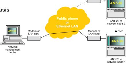
connected to a protected monitor point (PMP). By using test point scanners at the nodes, it is possible to connect a single ANT-20 to multiple PMPs. Via remote operation, a user at a network management center can now connect to each ANT-20.
