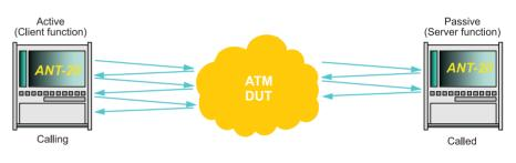
In *Called* mode, the ANT-20 with the BAG module can accept up to four calls simultaneously. Test scenarios involving five ANT-20/BAGs are thus possible.
